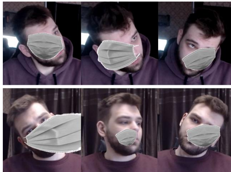
Fig. 2. Examples of incorrect generation of synthetic face images with overlaid PPE, obtained using MaskTheFace.
