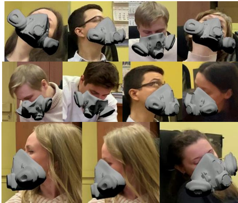
Fig. 14. Examples of incorrect PPE imposing according to criteria (1), (2) and (3), respectively.
